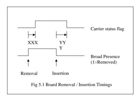
Fig 5.1: approximate time-state diagram of a carrier card removal and reinsertion event. There is a time delay when using polling to determine removal and reinsertion events, marked as XXX for removal and YYY for reinsertion. The delay marked XXX can affect system integrity if a driver attempts to access a carrier after it has been removed, but before this has been detected by the carrier polling task.
